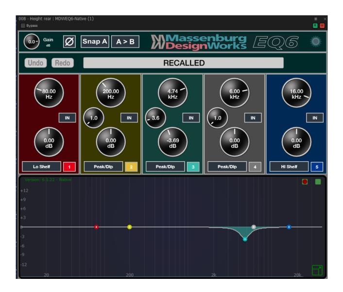
DSP, Lfe1 (Perc) has been low-pass filtered at 55 Hz 24dB/octave. Lfe2 (Double Bass) has been low-pass filtered at 65 Hz 24dB/octave.
