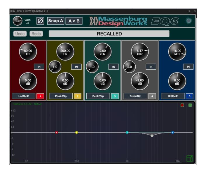
DSP, height front microphones: These microphones had both the black diffuse field grid and the APE50 that made for a somewhat brittle spectral character. This EQ emulates «undo» and seek to reset to what a DPA 4006 with regular grid and without the APE could have sounded like. EQ 9kHz 1.4Q -5dB
