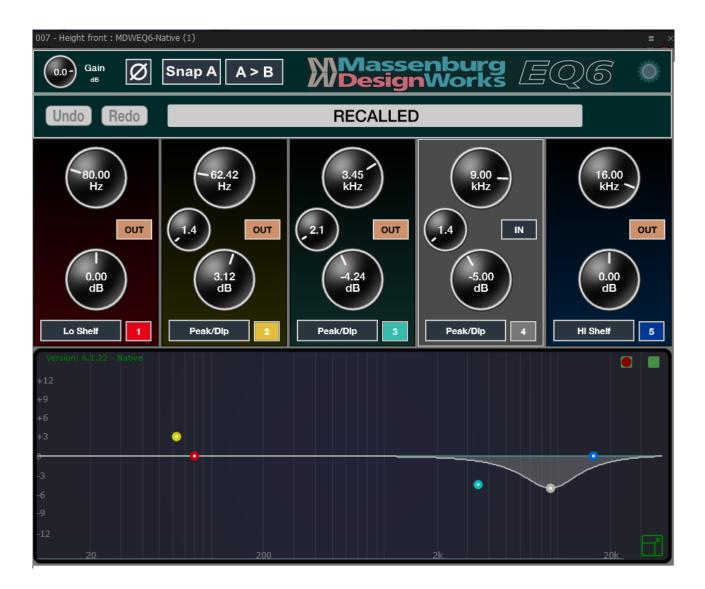
DSP, height rear microphones: These microphones had the APE50 that made for a somewhat brittle spectral character. This EQ emulates «undo» and seek to reset to what a DPA 4006 without the APE could have sounded like. EQ 4.74kHz 3.6Q -3.69dB. This EQ also limits the impact of the elevated THD of the faulty left rear height microphone.
