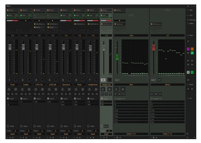
DSP, Rear microphones in bed: The rear pair 4041-S is pointing directly to the string instruments for maximum on-axis response. In a regular recording session I would have shifted the angle upwards to smoothen the texture. To simulate a slight off-axis response of the 4041-S an EQ 6.17kHz 2Q -1.6dB has been applied.
